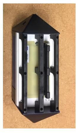
The conductivity sensor is a coated glass three electrode oscillator-based sensor similar to conductivity sensors from Sea-Bird Electronics.
