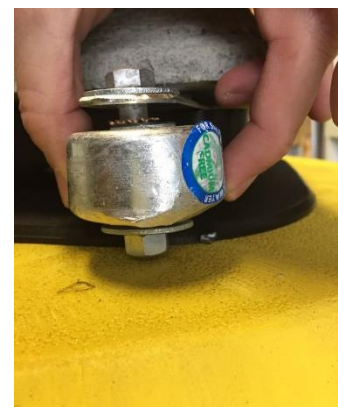
Figure 5 Anode installation side view
