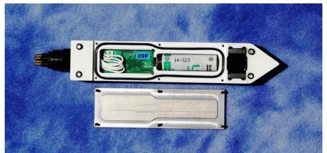
Ulti-modem with titanium battery cover removed
