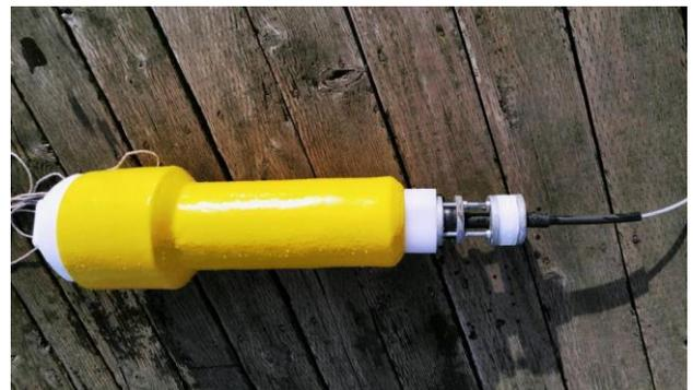
Buoyancy is adjusted to suit payload and expected wave conditions by varying the number of stacked weights on the tail section. Larger hull sizes are available to support larger payloads and/or deeper moorings and more dynamic environmental conditions.
