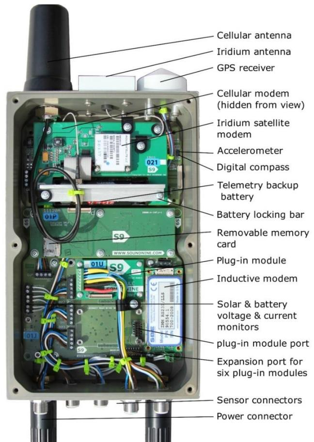
DANTE Buoy Controller (cover removed)
